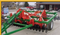
GLENCOE 7 SHANK SOIL SAVER spring shanks and blades, 3" twisted, 5 bar spike harrow, new paint, nice $7,200
