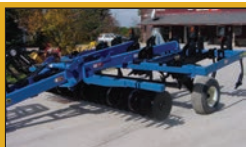
DMI ECOLO-CHAMP 1300 11 shank, 6 parabolic shanks and 5 chisel shanks, new steel, hydraulic gang adjust, excellent machine $14,500
