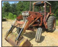
IH 1086 w/ IH 2250 loader, ROPS,dual hyd, dual pto, non running condition, inj pump bad? selling AS/IS. good parts or project. ....$4500.
