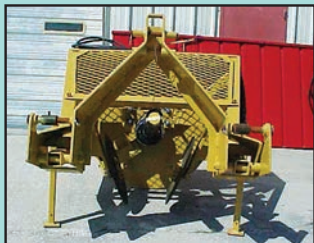
Toreq 3 Pt PTO Ditcher, 40" Wheel, Coulters, 540 or 1000 PTO Cat 2 or 3..... $8,500
