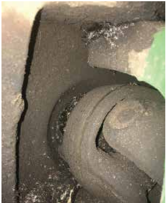
This MFWD input drive shaft has a leaky seal. Examine the constant velocity drive unit and the seals on the outboard drive and axle.
